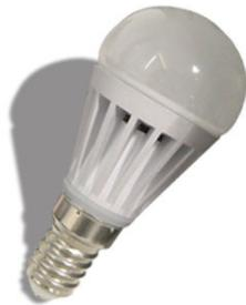
A40 4W LED bulb is designed and manufactured to replace the 25W incandescent /Halogen bulb and 7W CFL, the superior SMD LED solution and purity aluminium material makes the luminous efficacy high to 77LM/W, it is of excellently heat managed by conjoint structure which maintains the housing surface temperature under **69.3°C**, and LED joint temperature under **83.3°C**
