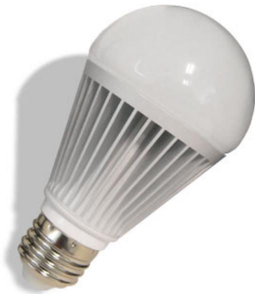
A60 7W LED bulb is designed and manufactured to replace the 40W incandescent /Halogen bulb and 15W CFL, the superior SMD LED solution and purity aluminium material makes the luminous efficacy high to 80LM/W, it is of excellently heat managed by conjoint structure which maintains the housing surface temperature under **57.1°C**, and LED joint temperature under **61.8°C**
